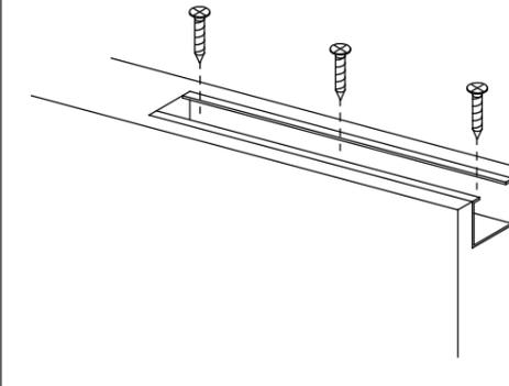
FIXER LE RAIL EN ALUMINIUM A LA PORTE AVEC LES VIS 4X30 FOURNIES. VERIFIER QUE LES VIS N'EMPECHENT PAS LE PASSAGE DE L'ETRIER.
